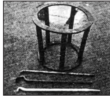
9. Mounting stand, used when mounting tires on rims that have been removed from a vehicle.
