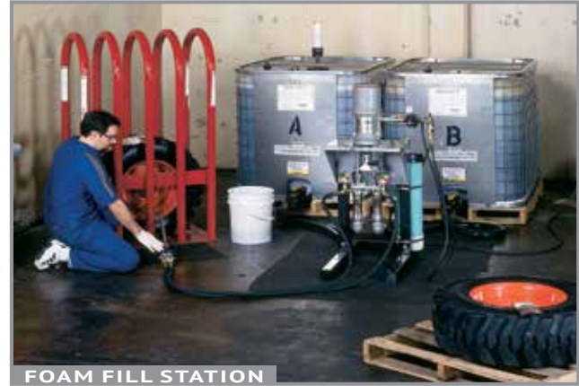
FOAM FILL STATION
